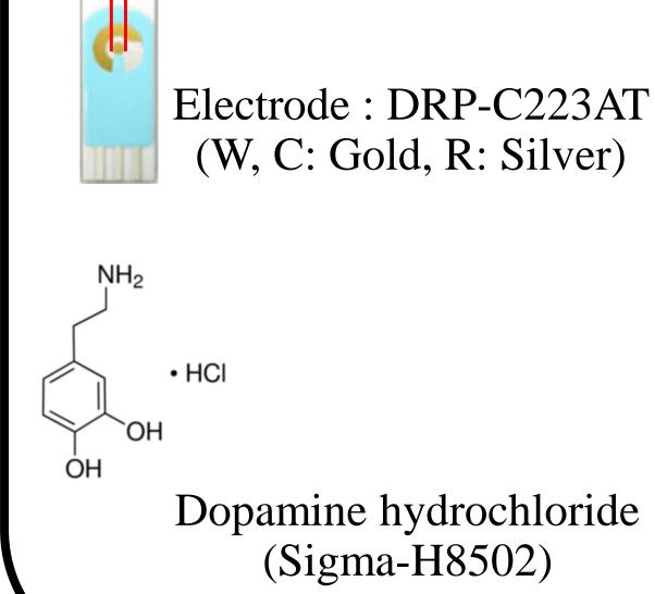
synthesized Poly(dopamine) was via cyclic voltammetry (-0.5 ~ 1.1 V, 30 cycles, 100 mV/s) with 20 mM dopamine in DI water. Synthesized polydopamine was observed by optical microscopy, AFM, and FIB-SEM.
